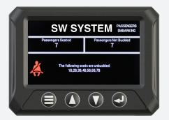
**UNBUCKLED PASSENGER COUNT DISPLAY** makes the driver aware of the count of passengers who are not buckled and where they are located within the vehicle.
