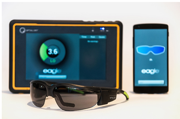
Figure 4. Optalert drowsiness detection glasses and eagle detection systems 29
