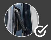
CABLING The cables are routed along the vehicle's body and into the cab.
