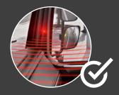
INSTALLATION OF THE WARNING SYSTEM The buzzer and light are mounted on the A-pillar.
