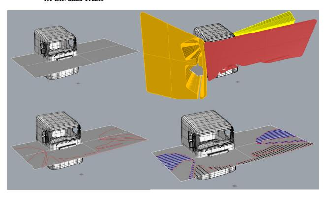
Figure 5 Visible Line Lengths to Each Side Based on an Example Intended for Left-Hand Traffic
